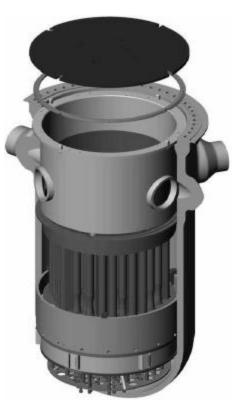
Figure 7-1 Maine Yankee RPV and Internals Prior to Segmentation
